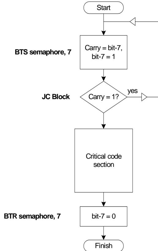
Here is a possible scenario, using two execution threads named **Thread-1** and **Thread-2**. They both need to execute the instructions in the critical code section, but they must not be permitted to enter the section at the same time. We assume here that a preemptive multitasking operating system is used, causing each thread to automatically be interrupted by the OS kernel on a regular basis:
